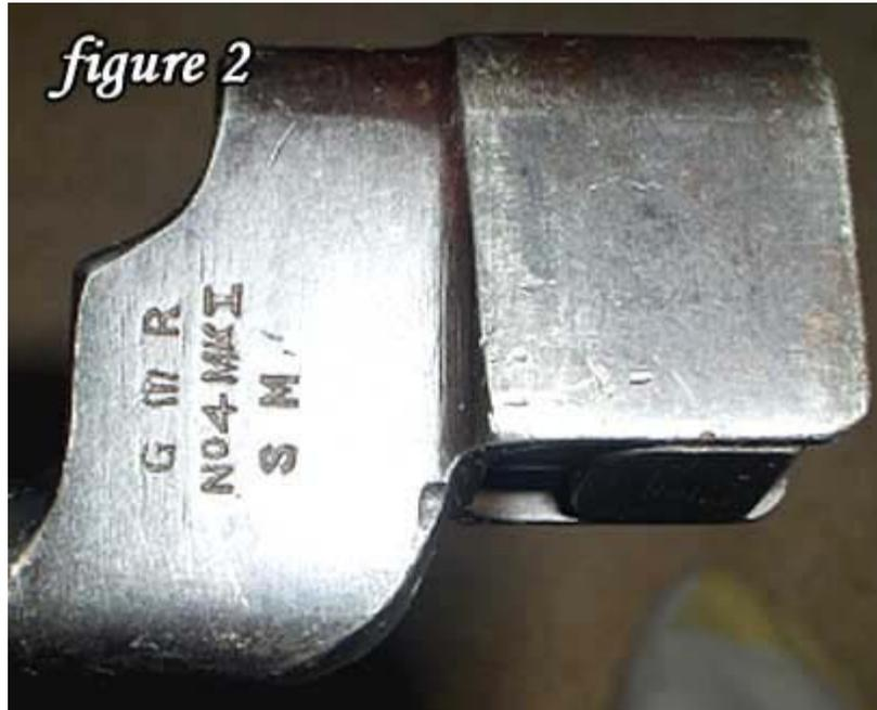
Note the nicely finished socket with deeply struck markings, including the royal cipher of King George VI. The workmanship that went into these early bayonets stands in stark contrast to the increasingly crude manufacturing practices exhibited by the Mk. II, Mk. II\* (pronounced, mark two star), and Mk. III bayonets that followed.
